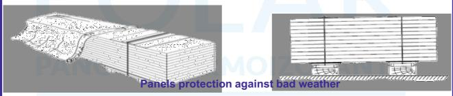
Panel positioning shall have a minimum 3 % - 5 % slope, for water flowing down purposes.
